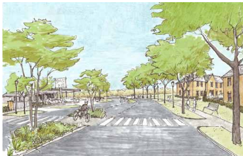
Mid-block pedestrian crossing with median refuge
