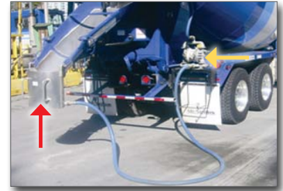
Figure 8. Chute washout bucket and pump
