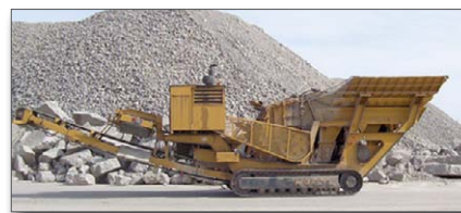
Figure 6. Crushed concrete stockpile and crusher
