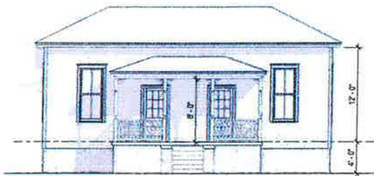
EAST/FRONT ELEVATION (new roof, columns, railings)
