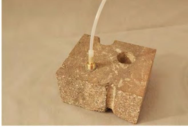
FIGURE 2 Vapor Pin™ Tubing Set-up
