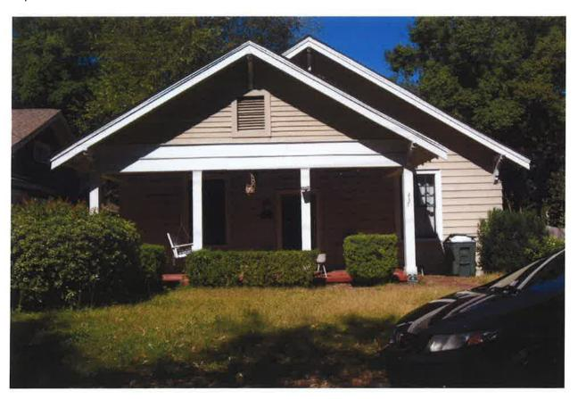
One story cross gable bungalow with pent roofs with secondary gable projections at each end with partial cornice returns; asymmetrical façade; 6:6 wood windows; 15 lite wood front door with 3 lite transom; front gable features pent roof, supported by grouping of 3 square posts on brick piers at corners with no intermediate supports; wood drop siding and frieze band under eave. C
