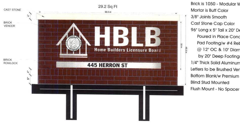
Brick is 1050 - Modular Wakefield Mortar is Buff Color 3/8" Joints Smooth Cast Stone Cap Color 96" Long x 5" Tall x 20" Deep Poured in Place Concrete Pad Footing/w #4 Rebar @ 12" OC & 10" Diameter by 20" Deep Footings 1/4" Thick Solid Aluminum Lettering Letters to be Brushed Vertical Bottom Blank/w Premium Vinyl **Blind Stud Mounted**
