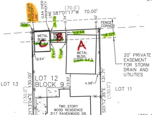
BASIS OF BEARING: THIS SURVEY HAS BEEN ROTATED TO MATCH THE STATE PLANE COORDINATE SYSTEM (ALABAMA EAST REGION)
