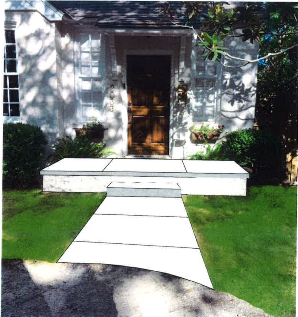
New Concrete Stoop and Walkway
