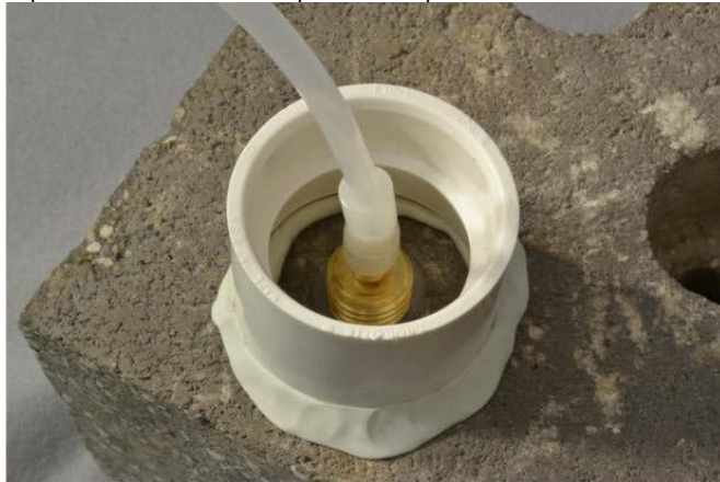
FIGURE 3 Vapor Pin Water Dam Set-up for Stick-up Installations
