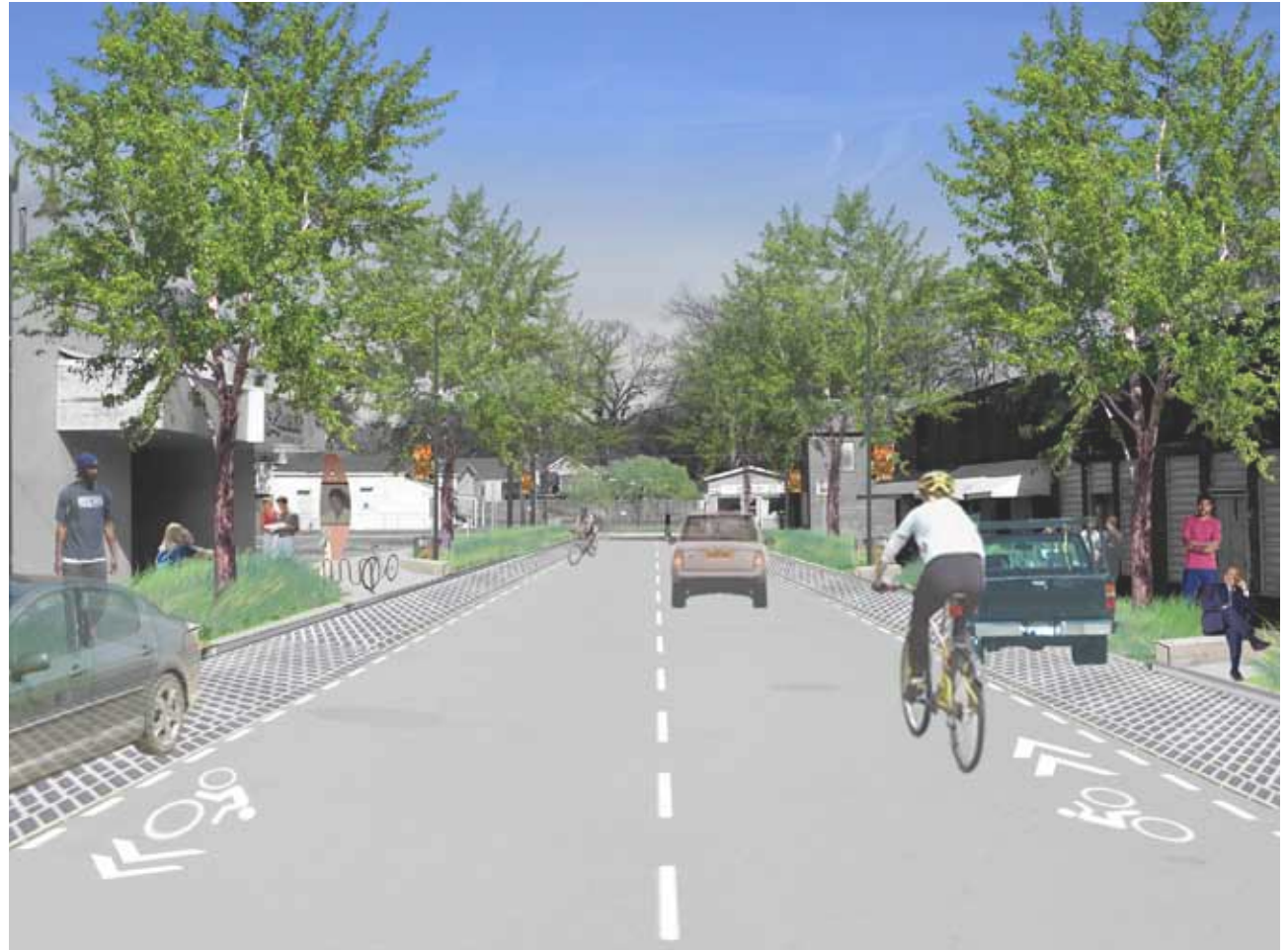
Figure 36: Design concept of stormwater planters, sharrow, and permeable paving in parking lane.
