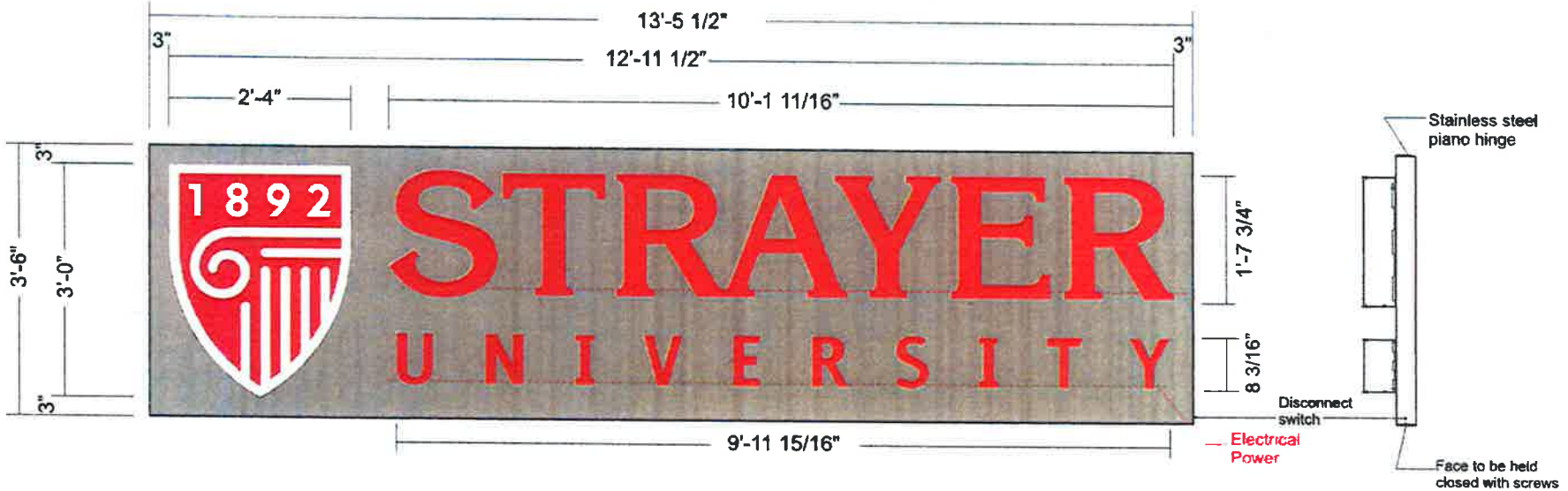
ILLUMINATED LETTERSET LAYOUT (STACKED VERSION W/ SHIELD) QUANTITY - 1
