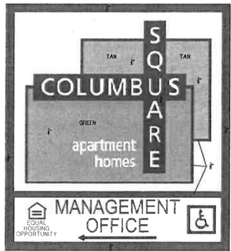
UNLESS OTHERWISE NOTED, SHADED AREAS ARE GRAY. 1" - INDICATES RAISED THICKNESS ABOVE BACKGROUND. ALL LETTERS ARE RAISED 1/2" ABOVE ADJACENT SURFACE. GRAPHIC FACING NORTH SCALE: 1/2"=1'-0"
