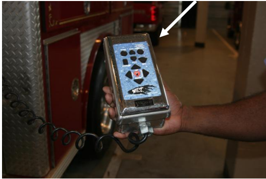
Pump Panel Control
