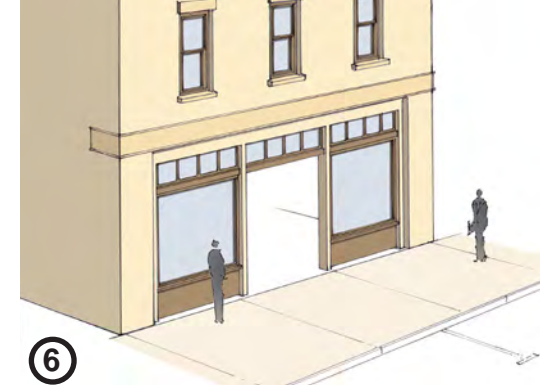
⑥ Cased windows sit atop knee-height bulkheads
